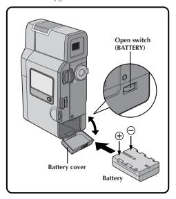
**OPEN BATTERY COVER**Slide down the open switch.
